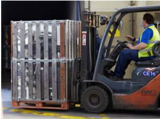
Picture 15. Example of container for WEEE containing LBs [43].
