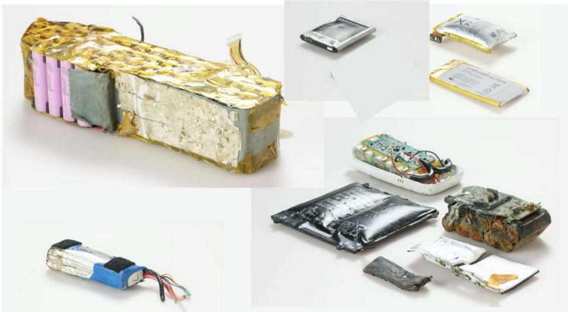
Picture 4. Examples of damaged batteries (Source: INOBAT).
