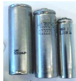
Picture 3. LBs missing the casing (naked).
