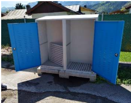
Picture 16. Left: protective housing for barrels containing LBs (Source MWE); Right: Cage for small WEEE containing integrated batteries (Source: EAK Austria).
