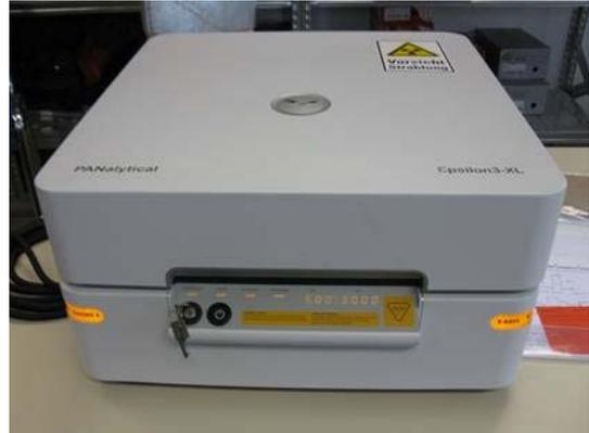
**The easiest method for using the XRF as screening method** is when the WEEE plastic recyclers apply this on the PCR plastic end-product, in other words at the end of the recycling process.
