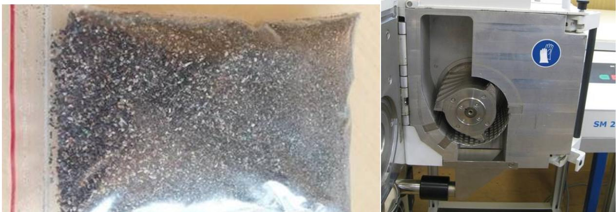
3. The dust sample again needs to be reduced in volume until you have the volume to press an “analysis tablet”
