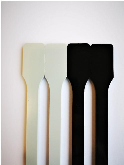
The screening method using XRF is generally applied by WEEE plastic recyclers on their end-products. The PCR flakes from WEEE are typically blended before and/or during the extrusion process, so that this final product will have been homogenized. Measurements are taking place typically on test-bars.
